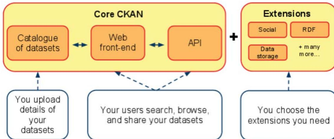
Figure 1. Overview of CKAN IT architecture highlighting the main functionalities provided. Source: Open Knowledge Foundation <https://goo.gl/L1nYzo>
