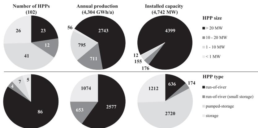
Figure 2. Number, annual production and installed capacity of hydropower plants (HPPs) size classes and types
